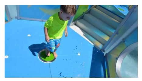
Another example of reducing water usage can be found in the water play zones. Instead of having water running and spraying the whole time, you can install "cause and effect" features where children can activate a water jet or a tipper with their hands or feet. (Bonus: This increases the play value.)
